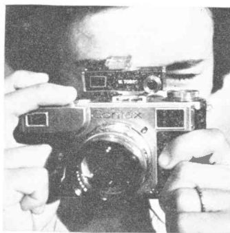
The Contameter is moved back and forth until the subject is in focus.
